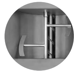
Bras de mélange TX32 ML / Minimix 98 Mixing arm TX32 ML / Minimix 98
